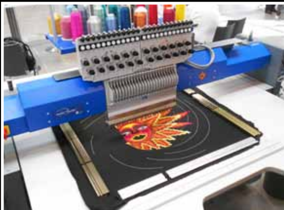
RACER 1 XL with 24 needles and a working area of 700 mm x 700 mm
