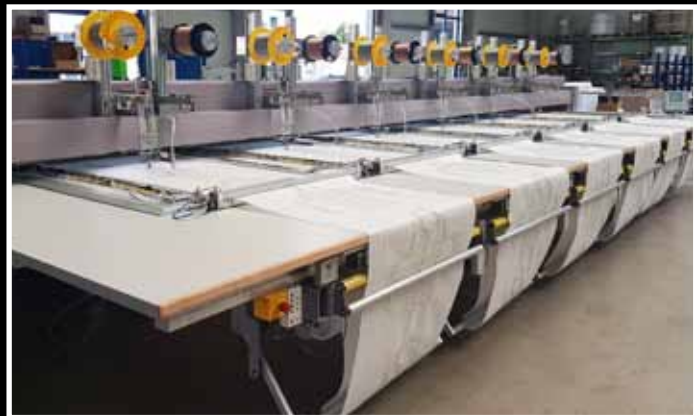
Automatic Car Seat Heating Production on a ZSK YCW 0600 with 6 Production Units.
