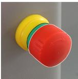
4 to 8-head machines are equipped with additional, separate **EMERGENCY STOP buttons**.
