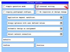
Switch on the function *Writing*. Starting from the basic screen of the T8 control unit, press the following buttons:
