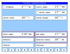
The setting dialog *Circular counterclock-wise* is used to adjust the settings for circular monograms. The same functions apply to this setting dialog as to the setup dialog *Singleline*. In addition, the *Start angle*, the *End angle* and the *Baseline radius* can be adjusted here.
