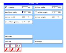
When the input fields are marked, the dialog display switches over and the buttons **[U1] - [U3]** are displayed.
