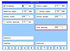
The setting dialog *Multiline* is used to adjust the settings for multiline monograms. The same functions apply to this setting dialog as to the setting dialog *Singleline*. In addition, the *Line spacing* between the lines can be adjusted here.
