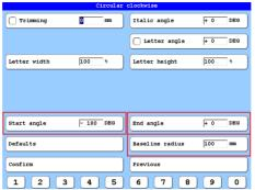
The setting dialog *Circular clockwise* is is used to adjust the settings for circular monograms. The same functions apply to this setting dialog as to the setup dialog *Singleline*. In addition, the *Start angle*, the *End angle* and the *Baseline radius* can be adjusted here.
