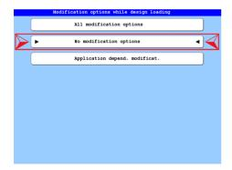
If the button *No modification options* is active, the modification dialog will be switched off and will not appear when loading a design.
