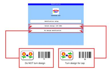
The design is loaded, modified, optimized and assigned to the embroidering machine according to the selection.
