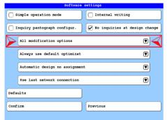
Switch on the function *All modification options*. Starting from the base screen of the T8 control unit, press the following buttons:
