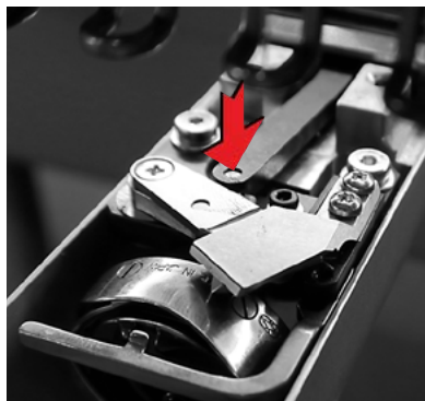
Fig. 9: Cylinder arm, connecting rod lubrication points
