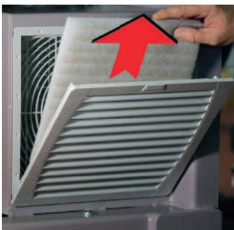
Withdrawing filter element
