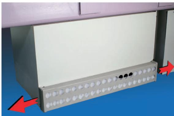
Carbon protection Machines Series L-Z (Filter change)
