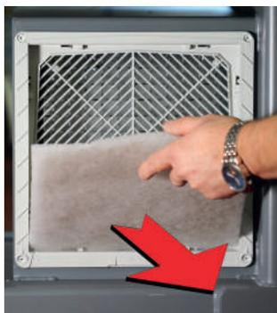
Withdrawing filter element
