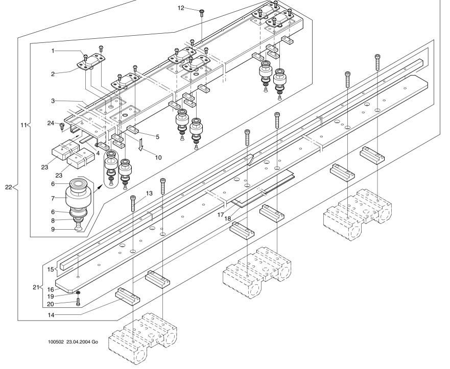
Maschinentype: Flachbettstickmaschine Baugruppe: Connection for pantograph and pantograph drive - Seitliche Pantographenanbindung SCF
