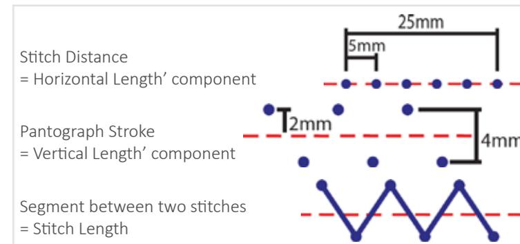
Figure 6 – Parameters to determine the ZigZag Stitches
