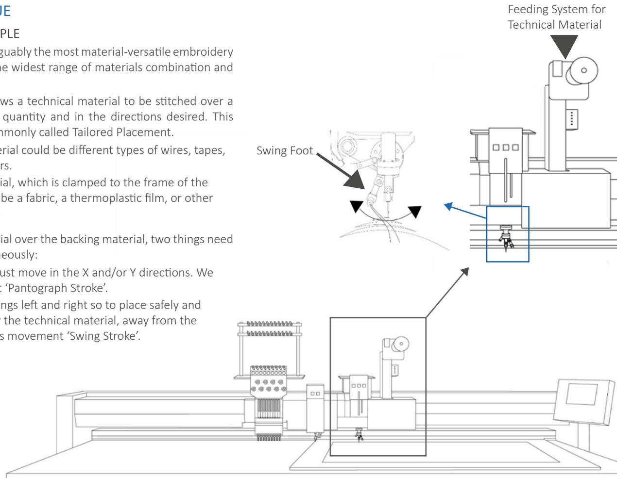
Figure 4 – Overview and Key Parts for the W-Head
