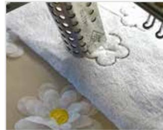
Fig 21 – Hot Air Cutting Device
