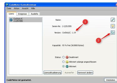
The EPCwin version 5.x requires firmware version 1.14 and higher. You will find your current version of firmware in the centre of the dialogue (arrow 1). If the shown version is less than 1.14, you have to carry out an update of the firmware.
